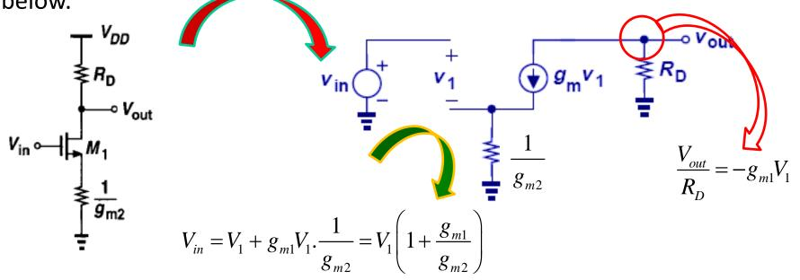
**Simplification gives:**  $V_{out} = -g_{m1}V_1R_D$
