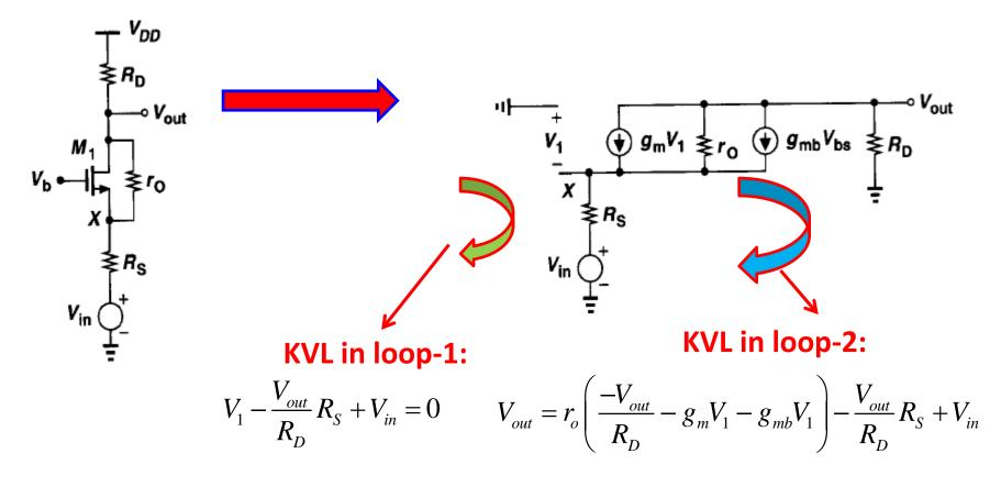
• Simplification gives:  $\frac{V_{out}}{V_{in}} = A_v = \frac{(g_m + g_{mb})r_o + 1}{r_o + (g_m + g_{mb})r_oR_s + R_s + R_D}R_D$
