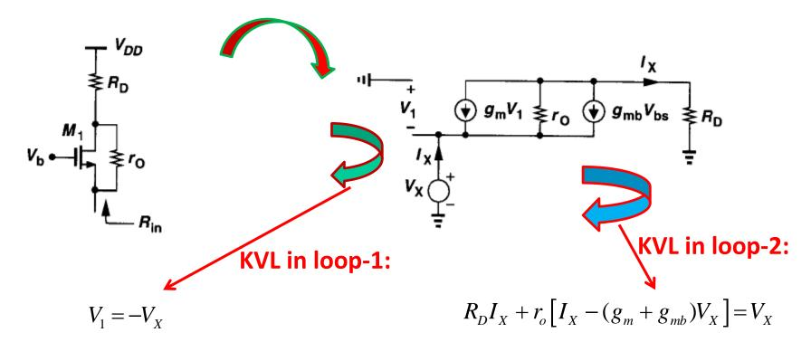
$$R_{in} = \frac{V_X}{I_X} = \frac{R_D + r_o}{1 + (g_m + g_{mb})r_o} \approx \frac{R_D}{(g_m + g_{mb})r_o} + \frac{1}{(g_m + g_{mb})r_o}$$
