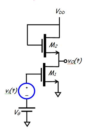
**Q:** What is the small-signal open-circuit voltage gain, input resistance, and output resistance of this amplifier?
