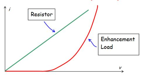
Therefore, we can build a common source amplifier with either a resistor, or in the case of an integrated circuit, an enhancement load.
