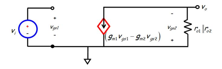
• We find that:  $V_{gs1} = V_i$   $V_{gs2} = -V_o$
