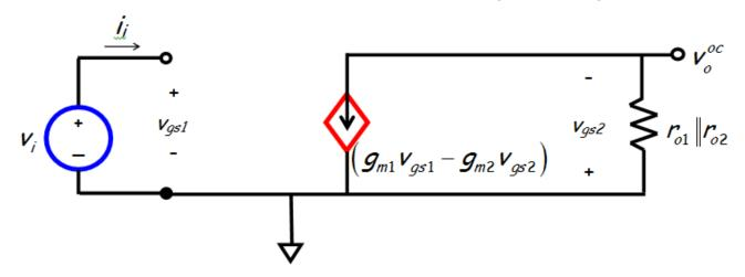
Now for the output resistance, we know that the open-circuit output voltage is:
