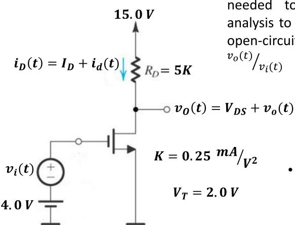
Lets look at the last example. You needed to perform a small-signal analysis to determine the small-signal open-circuit **voltage** gain  $A_v = \frac{v_o(t)}{v_i(t)}$
