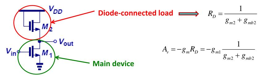
$$\Rightarrow A_{v} = -\frac{g_{m1}}{g_{m2}} \frac{1}{1+\eta} \qquad \qquad \eta = \frac{g_{mb2}}{g_{m2}} \qquad \qquad \therefore A_{v} = -\frac{\sqrt{2\mu_{n}C_{ox}(W/L)_{1}I_{D1}}}{\sqrt{2\mu_{n}C_{ox}(W/L)_{2}I_{D2}}} \frac{1}{1+\eta}$$
