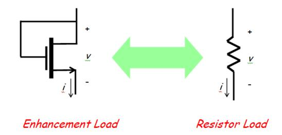
Q: How does this "enhancement load" resemble a resistor?
