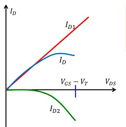
It is apparent that the second term  $I_{D2}$  works to **reduce** the total drain current from its "**resistor-like**" value  $I_{D1}$ . This of course is physically due to the **reduction in channel conductivity** as  $V_{DS}$  increases.
