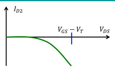
Moreover, the minus sign means that as  $V_{DS}$  increases,  $I_{D2}$  will actually **decrease!** This behavior is **nothing** like a resistor—what the heck is going on here??
