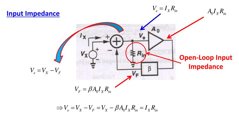
$$\therefore R_{in,closed} = \frac{V_X}{I_X} = R_{in} (1 + \beta A_0)$$
