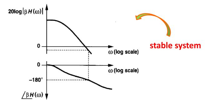
To make the system stable, the idea is to minimize the total phase shift so that for |βH|=1, <βH is still more positive than -180<sup>0</sup>
