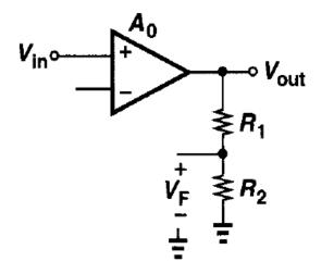
For voltage sensing – parallel to the output node of this differential input but single ended output amplifier
