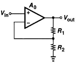
The voltage signal from feedback network is fed to the other input node of the differential amplifier
