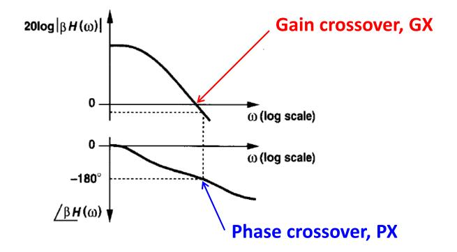
If  $\beta$  is reduced (i.e., less feedback is applied), the magnitude plot will shift down  $\rightarrow$  essentially moves GX closer to origin  $\rightarrow$  in turn makes the system more stable
