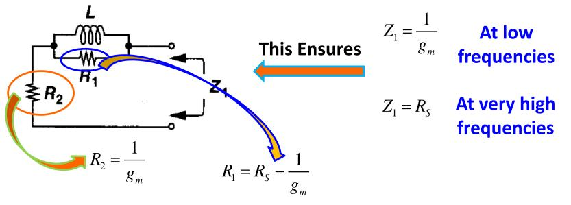
• For the determination of <u>L</u>, equate the Z<sub>1</sub> expression to that of Z<sub>out</sub>
