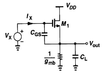
$$V_X = \frac{I_X}{C_{GS}s} + \left(I_X + \frac{g_m I_X}{C_{GS}s}\right) \left(\frac{1}{g_{mb}} \| \frac{1}{C_L s}\right)$$
