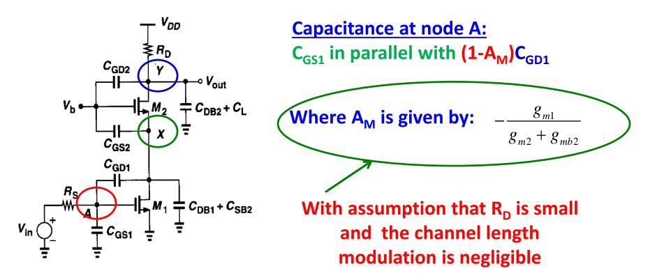
For equal dimensions of  $M_1$  and  $M_2$ :  $A_M$  approximately equals  $1 \rightarrow$ therefore  $C_{GD}$  gets multiplied by a factor of roughly 2 both at node A as well as at node X  $\rightarrow$  much smaller multiplication factor as compared to a single CS stage
