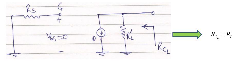
Thus, the effective time constant:  $\tau_H = C_{GS}R_{GS} + C_{GD}R_{GD} + C_LR_{C_L}$
