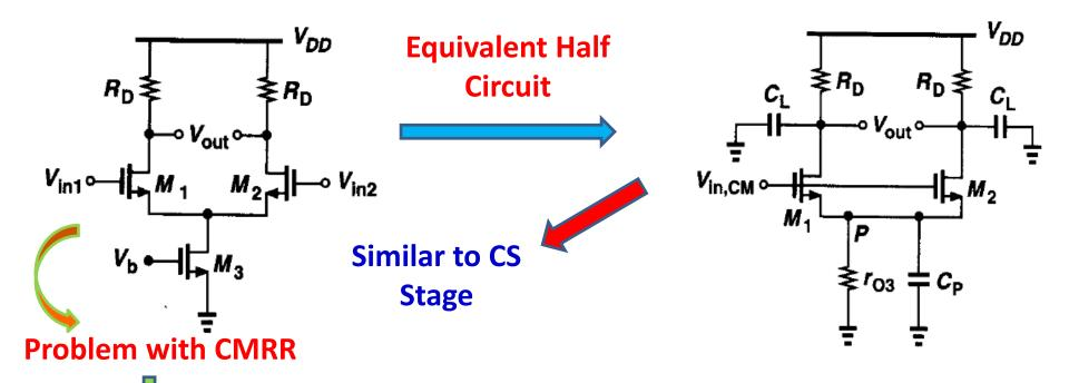
To minimize voltage headroom consumed by  $M_3 \rightarrow its$  width is maximized  $\rightarrow$  increases the capacitance contribution by  $M_3 \rightarrow$ higher capacitance at the source of  $M_1$  and  $M_2 \rightarrow$  degrades the differential gain of  $M_1$  and  $M_2$  at high frequencies  $\rightarrow$  reduces the CMRR at high frequencies
