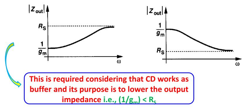
The output impedance increases with frequency ↔ clear indication of the presence of inductive element
