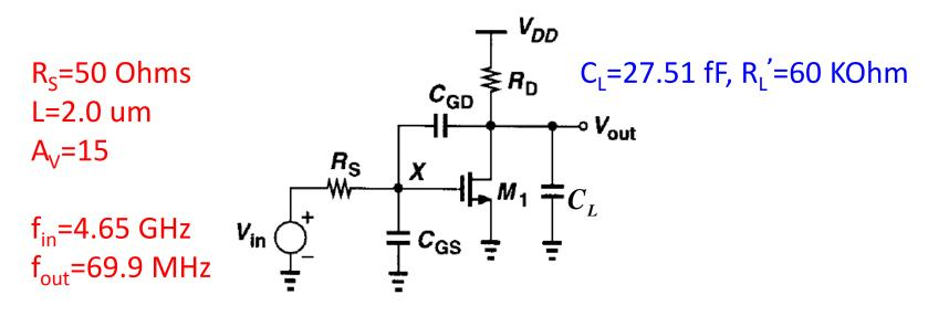
$$\omega_{in} = \frac{1}{R_{S} \left( C_{GS} + \left( 1 + g_{m} R_{L}^{'} \right) C_{GD} \right)} \qquad \qquad \omega_{out} = \frac{1}{R_{L}^{'} \left( C_{L} + C_{GD} \right)}$$
