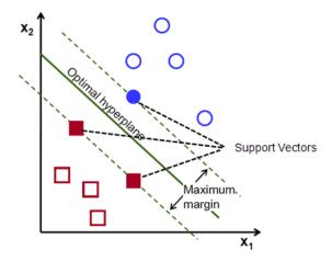
Fig. 2.7 Support Vector Machine classifier with a optimal hyper-plane separating the two classes.
